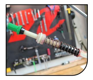
Thread a piston removal tool (or a long M6 bolt as seen in the bottom photo) into the air piston and remove it from the stanchion. Once the piston is removed clean the inside of the stanchion with isopropyl alcohol and a lint free towel. Inspect the inside and outside of the stanchion for scratches or other damage.
