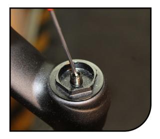
Remove air cap using a 20mm socket.
