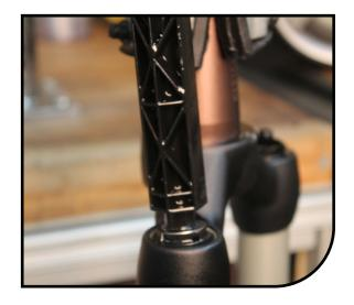
If installing an ABS+ damper use a 24mm socket and torque wrench, tighten the damper to 60–80 in lbs [6.8–9.0 NM]. If installing a Kwik Toggle damper use a 1" socket or crow's foot, the cassette tool, and a torque wrench to tighten down the damper to the same torque specification.
