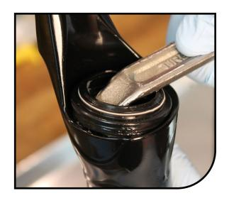
Remove old foam wiper rings. Apply semi-bath fluid to the new foam wiper rings and install into fork casting.
