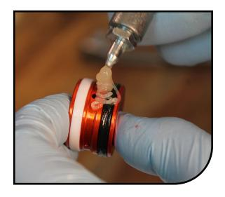
Install greased air piston into the top of the stanchion and push it down past the threads.
