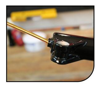
Using an 8mm hex wrench tighten the rebound damper rod and air spring assembly to 35–40 in lb [3.95–4.5 N m] by turning them **counter-clockwise.** Do not overtighten, doing so can damage the end of the rods.
