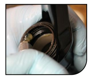
Fill the air chamber with a small amount of air (30-50PSI). This will extend the air spring assembly and make casting installation easier.
